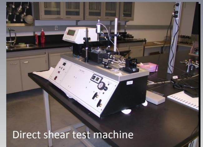
Direct shear test machine
